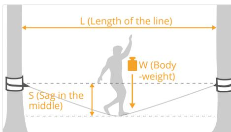
$$\frac{L (m) * W (kg)}{S (m) * 400} = \text{tension in kN}$$
